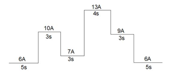
APM DC E-load could loaded according to edited waveform
